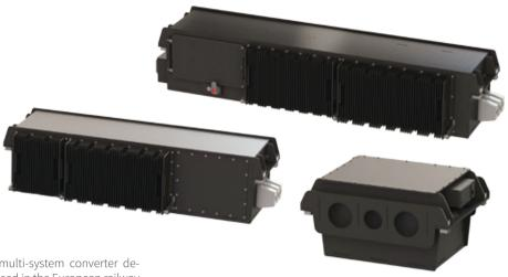
The PSM-50W4 static converter is a multi-system converter designed to convert DC and AC voltages used in the European railway traction, into 24 VDC, 3×400 VAC and 230 VAC, required in the low voltage systems of coaches.
