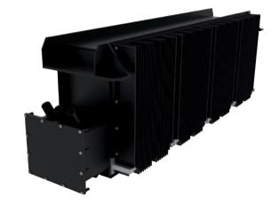
The PSM-3×8 static converter is designed to convert 110 VDC on-board voltage into three, regulated U/f 3×380 VAC outputs and one 24 VDC output required to power the loads installed in a passenger coach (compressors, air conditioning system fans, DC drives for doors).
