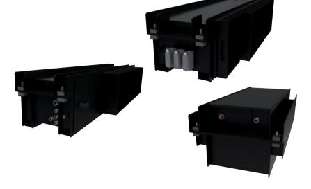
The PSM-50W static converter is a multi-system converter designed to convert DC and AC voltages used in the European railway traction, into 24 VDC,  $3\times400$  VAC and 230 VAC, required in the low voltage systems of coaches.
