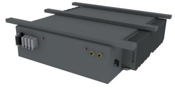
The PSM-50W static converter is a multi-system converter designed to convert DC and AC voltages used in the European railway traction, into 24 VDC, 3×400 VAC and 230 VAC, required in the low voltage systems of coaches.
