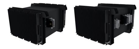
The PSM-45 static converter has been designed to convert 3000 V (DC or AC) used in the railway traction networks into 110 VDC and 24 VDC as well as  $3\times380$  VAC and 220 VAC, used in the low voltage
