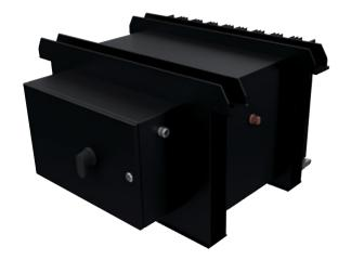
The PSM-6k5W static converter is a multi-system converter designed to convert DC and AC voltages from the railway traction networks, into 24 VDC, used in low voltage installations for coaches.
