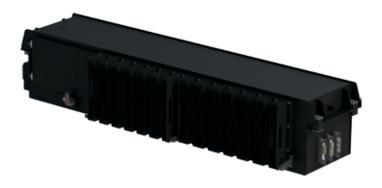
The PSM-12WB static converter is a multi-system converter designed to convert DC and AC voltages used in the European railway traction, into 24 VDC and 230 VAC, required in the low voltage systems of coaches.
