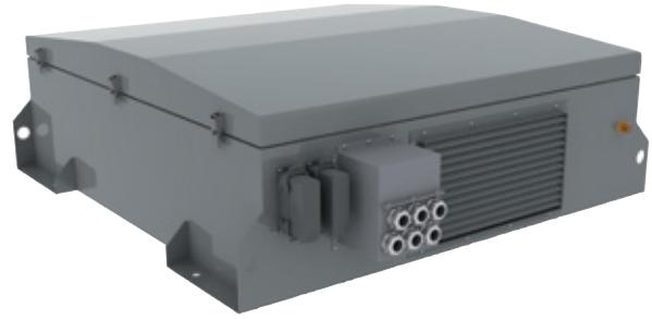
The PSM-60T auxiliary converter has been designed to convert DC voltage of the 600 VDC traction into 24 VDC voltage, as well as 3x400 VAC and 230 VAC voltage, needed to supply the auxiliary circuitry of the tram system, driver's air conditioning and car ventilation.
