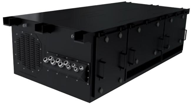
The PSM-132 auxiliary converter has been designed to convert DC voltage of the 750 VDC metro traction into 3×380 VAC 60 Hz AC voltage, applied in the low voltage systems of metro, used to supply the auxiliary circuitry in the metro system, air conditioning and DC loads.
