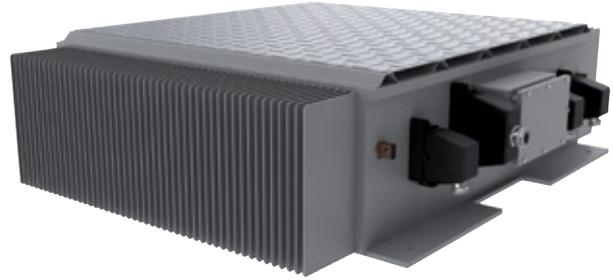
The PSM-30T auxiliary converter has been designed to convert DC voltage of the 600 VDC traction into 24 VDC voltage as well as into 3x400 V and 230 VAC voltage, needed to supply the auxiliary circuitry in the tram system, driver's air conditioning and car ventilation.
