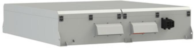
The FT-250-600/750 propulsion inverter is designed to power the traction motor, which drives the wheel axle of the trolleybus. The container that houses the FT-250-600/750 propulsion inverter together with the RWN-360-600/750 switchboard, PSM-52T auxiliary converter and FCEC-85 fuel cell converter, is to be mounted on the roof of the vehicle. The propulsion inverter is used for the traction power supply of 600/750 VDC.
