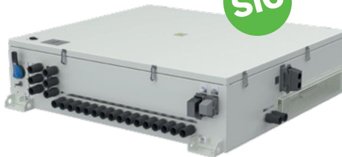
Propulsion inverter is designed to supply the motor or motors driving the wheels in an electric bus. Container of the inverter with HV switchgear and PSM auxiliary converter is designed for installation on the roof of the vehicle. Propulsion inverter is designed to be powered from the traction battery.
