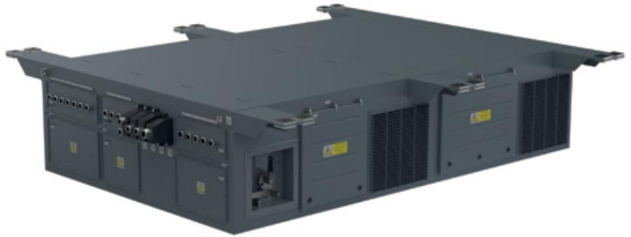
The traction container box is designed to power the traction motors driving the wheel axles in a metro vehicle. The device is designed for installation under the vehicle floor. Propulsion inverters are designed to be supplied by 750 VDC traction voltage. The drive units in the vehicle enable starting, driving with a given torque, coasting and braking the vehicle. They also enable starting, driving and braking with the set reverse travel direction.
