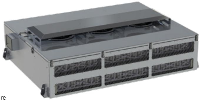
Energy recovery system UOE-02 with banks of supercapacitors are used to recovery LRV braking energy and storage them in supercapacitors. Storage energy is used to supply auxiliary circuit on LRV during stand or it is consumed by propulsion inverter during start-up of LRV. When emergency driving is required, energy stored in supercapacitors can be also consumed by propulsion system (eg. in case of no catenary voltage appearance).
