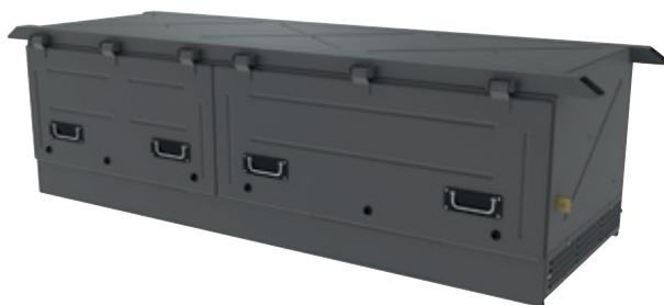
The auxiliary converter PSM-68 is a fully automated device designed for converting traction power supply 750 VDC voltage to 110 VDC voltage of auxiliary circuits, 3×400 V/50 Hz and batteries charging. The device uses the technique of multiple conversion of energy. 110 V output voltage is adjusted to the charge state of the battery cooperating with the converter so that the charging cur-
