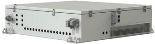
Propulsion inverter is intended to supply traction motor which drive the bus wheels. The inverter container with the RWN switchgear and PSM auxiliary converter is intended for installation on the vehicle roof.
